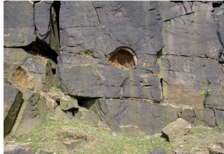
Patches of weak sandstone in Pule Edge Quarry, cemented by iron instead of quartz.
